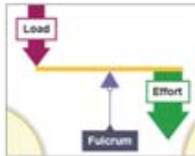
1 st Class Lever: Fulcrum in the centre E.g. Scissors
